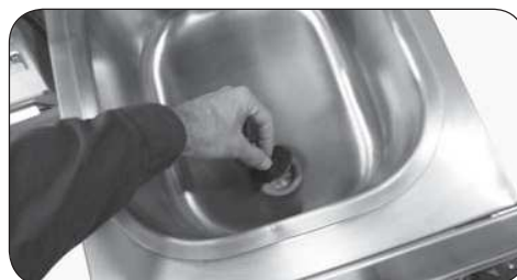
Fig. 8-2 Clean ice storage drain plug
