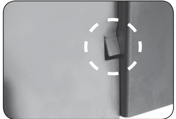
Fig. 19-2 Tab slightly bent in for clearance
