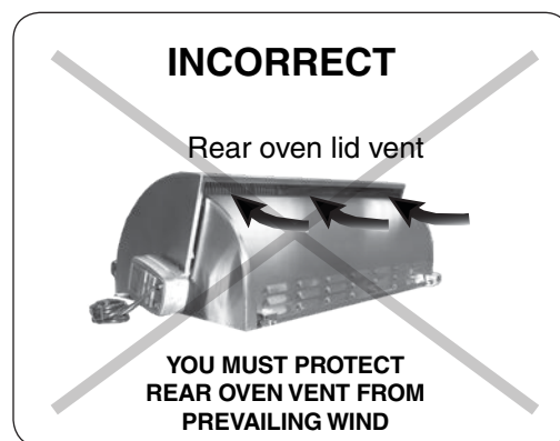
Fig. 10-3 Airflow direction - INCORRECT
