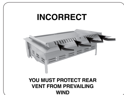
Fig. 12-3 Airflow direction - INCORRECT
