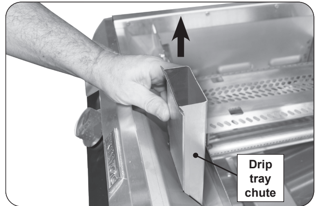
Fig. 40-2 Drip tray chute removal
